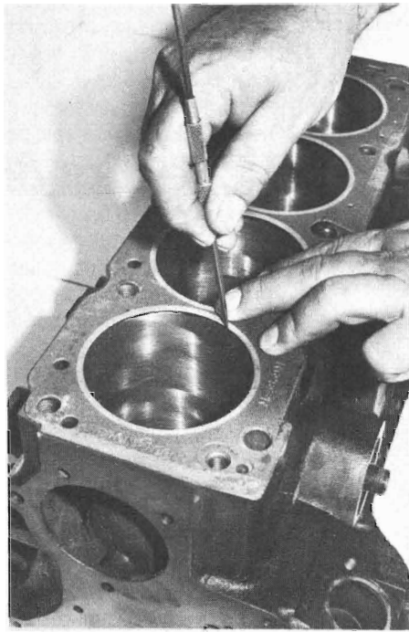
7-1. To O-ring the block, the first step is to blue the cylinder head deck face around the bores.
