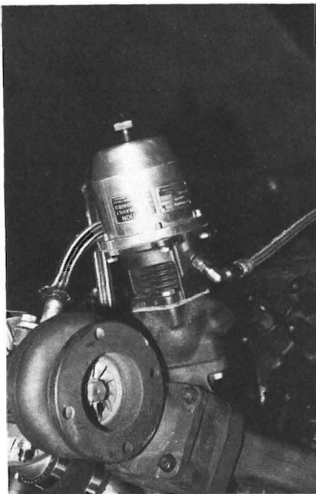
11-4. Waste gates come in many sizes, both big and small. There are numerous cheap (and nasty) waste gates on the market. Airesearch makes a good, though expensive, waste gate, an example of which is shown here. Another quality unit is produced by Environmental Products in Los Angeles.
