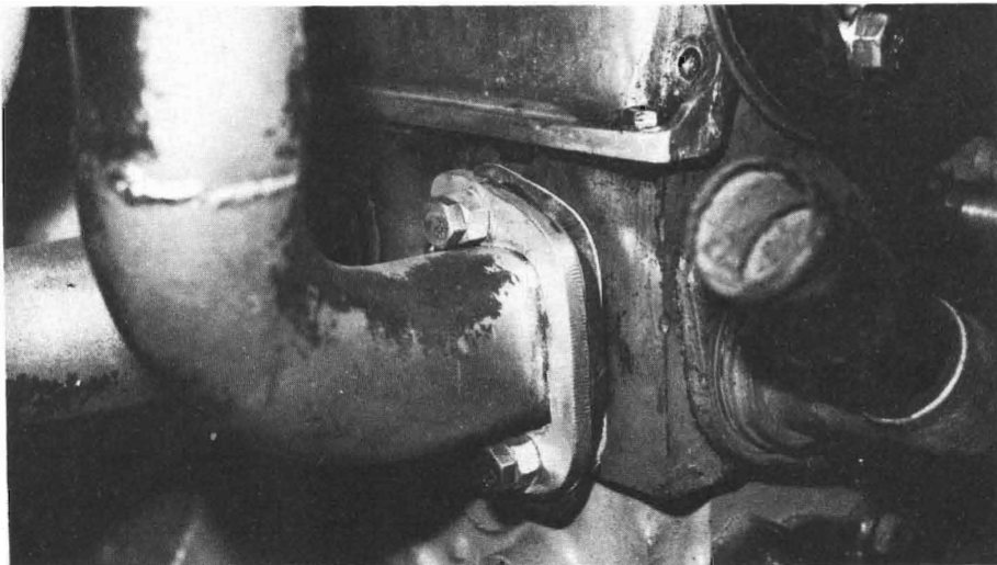
5-1. Here's the 2" diameter exhaust pipe used on the Vizard/Esslinger 2000 cc engine. Note the plate between the manifold flange and head. This plate . . .
