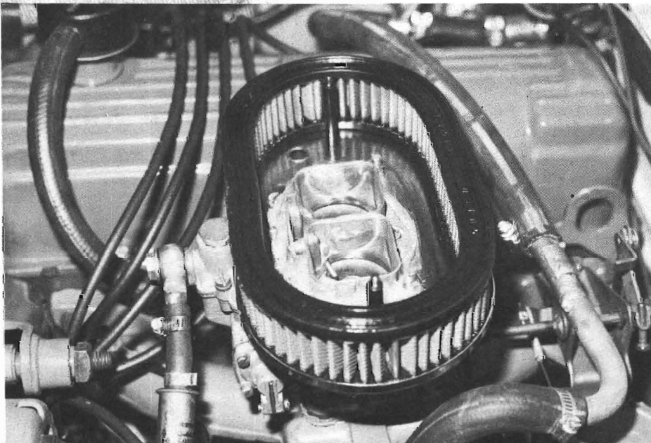
4-20. I tried a Weber 40D. F.I.5 Weber both in standard form and modified on a 2-litre Pinto. It produced good hp but there were many drawbacks as the test explains.
