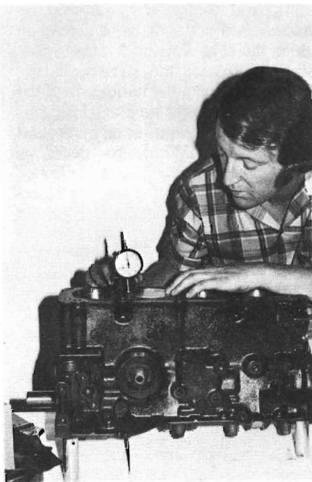
7-21B After selective assembly of pistons and rods, each rod and piston set can be checked out for compression height in the bore. This is just what I am doing in this shot here. I tried each rod and piston assembly in each bore. There is no need to put the cap on the rod when doing this check. As long as the crank is lubricated and you turn the crank to push the piston up to TDC, you will do fine. Make sure you always check the piston to deck clearance at a consistent spot on the piston and it must be above the centre-line of the crank, otherwise you will also measure a degree of piston rocking.
