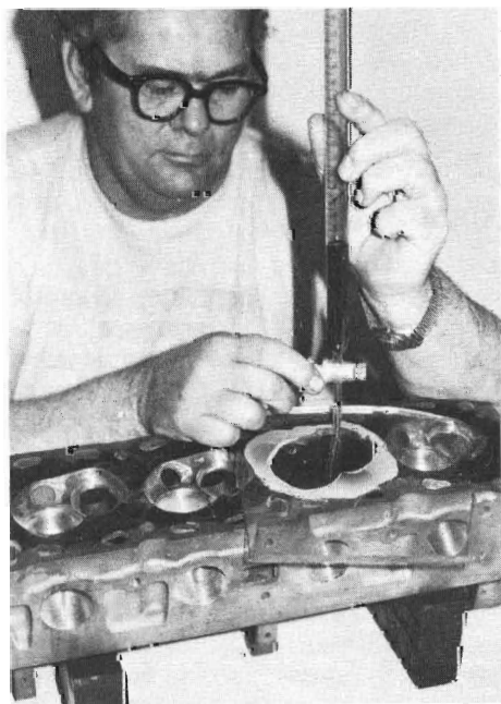
2-36. Smear grease around the edge of the chamber, then position the plastic sheet so that the holes are on the high side. This allows trapped air to escape while filling the chamber.
