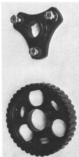
3-1. An adjustable cam sprocket is a wise investment any time a cam change is made. On occasions, the standard cam can be far enough outright from the factory to warrant using an adjustable sprocket for correction. Some adjustable sprockets will not clear the standard belt casing so check this out before you buy. Item shown here is made by Holbay.
