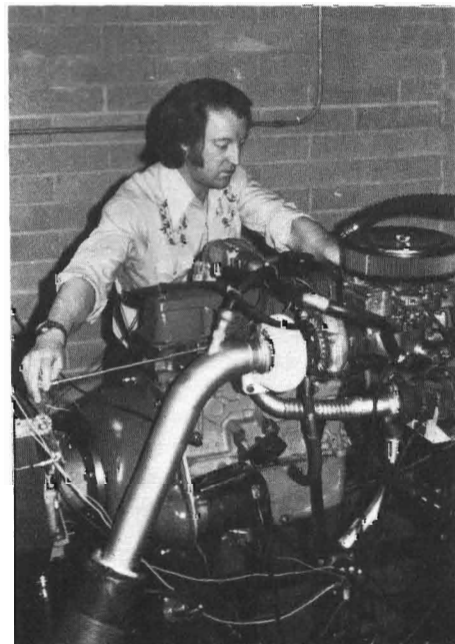
11-1. Here I am making some minor adjustments on the engine before a power run is taken. Note the white exhaust housing on the turbo. This is because it was finished with a coating of Heanium to retain the heat.
