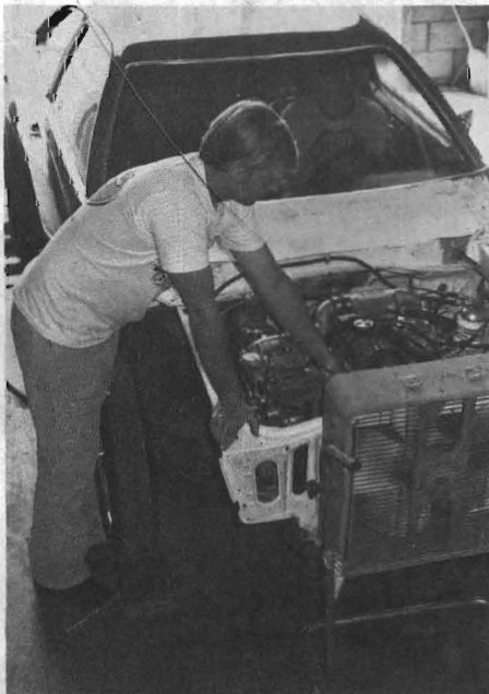
11-13. Jim Flynn's turbo pinto undergoes a full check out on the chassis dyno. Full power runs were not possible as the car would climb right off the rollers at about 150hp at the wheels. Unfortunately this power occurred at part throttle, just at the point when the engine came up on the cam. In spite of this, a great deal was found out about idle, transition and pump circuits. After dialling in these parameters, the car could be driven around just like an ordinary road car.
