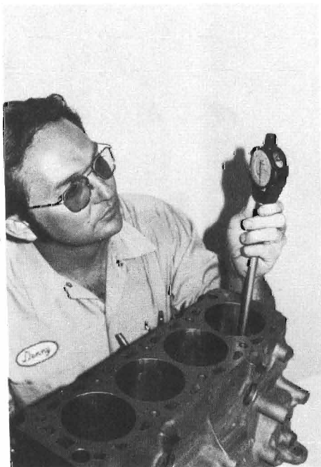
7-15. Here, Denny Wyckoff runs through the final stages of checking out a block for a hot street machine. Not only are the bores accurately sized but they have also been given the correct honing finish, as can be seen. The block has also been decked and a very important step, the tops of the bores have been chamfered to allow easy installation of the piston and ring assembly.
