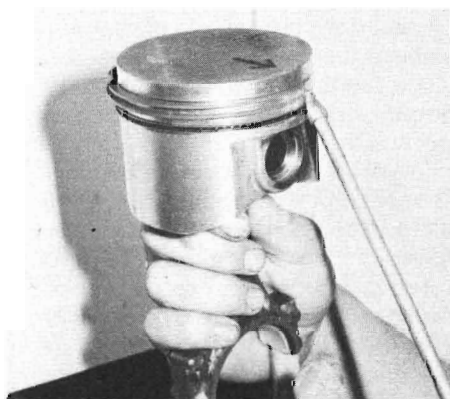
7-22. Here I am just installing a T.R.W. piston into a high performance street engine. The golden rule with the assembly of any engine is to give the rings adequate lubrication before installing them in the block. To make sure I put the piston in the right way, I mark a large arrow on the piston face, as can be seen here. Note that this T.R.W. piston has had the dome machined off it.
