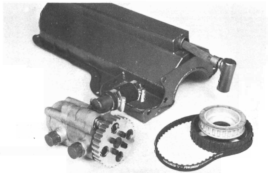
8-6. Here is a baffled anti-surge sump made for a road racer by Shankle Automotive. This pump was used together with a slightly repositioned pick-up pipe.
