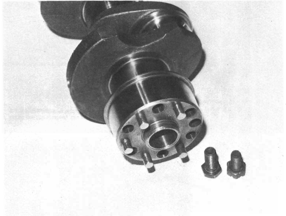
7-46. Here's the fix for flywheels parting company from crankshafts. A \frac{5}{16} " dowel between each bolt hole, that's the first reinforcement. Secondly each bolt hole in this instance has been drilled out and tapped to a larger scale size. The two bolts in the picture demonstrate the difference between the larger bolt used and the standard bolt.
